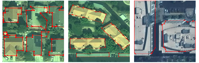
Figure 5: Three typical examples of failure cases of our proposed method. Our method fails to produce accurate polygons for buildings that are seriously sheltered by trees (left), buildings with multiple extremely short edges (middle), and high-rise buildings with serious parallax effect (right).
